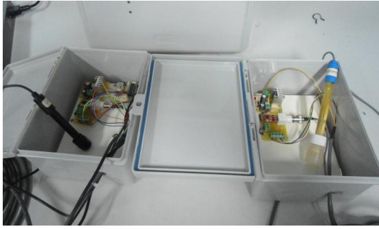
Fig. 3. pH and DO sensors, mounted in an IP 65 housing, with their own processing units.
