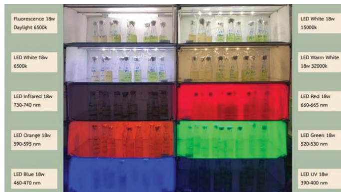
Figure 1 Different light wavelengths of white light Fluorescent bulbs (Color Temperature 6,500 K), warm white LED bulbs (Color Temperature 3,200 K), white LED bulbs (Color Temperature 6,500 K), white LED bulbs (Color Temperature 15,000 K), Infrared LED bulbs (730-740 nm), red LED bulbs (620-625 nm), Orange LED bulbs (590-595 nm), Green LED bulbs (520-525 nm), Red LED bulbs (620-625 nm), Blue LED bulbs (460-465 nm) and UV LED bulbs (390-400 nm).
