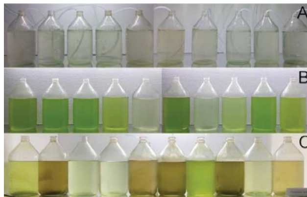
Figure 2 Growth of Chlorella sp. under difference Light sources condition of white light Fluorescent bulbs (Color Temperature 6,500 K), warm white LED bulbs(Color Temperature 3,200 K), white LED bulbs (Color Temperature 6,500 K), white LED bulbs (Color Temperature 15,000 K), Infrared LED bulbs (730-740 nm), red LED bulbs (620-625 nm), Orange LED bulbs (590-595 nm), Green LED bulbs (520-525 nm), Blue LED bulbs (460-465 nm) and UV LED bulbs (520-525 nm) at starting the experiment (A), 5 days (B) and 10 days (C).
